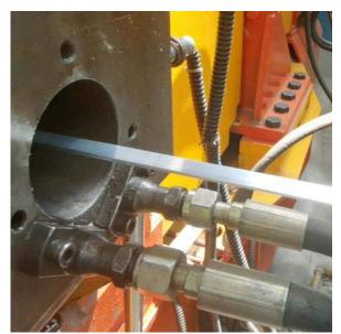
Bare wire annealing. Annealing is a process at high temperature which aim to soften the copper and make it more malleable.
